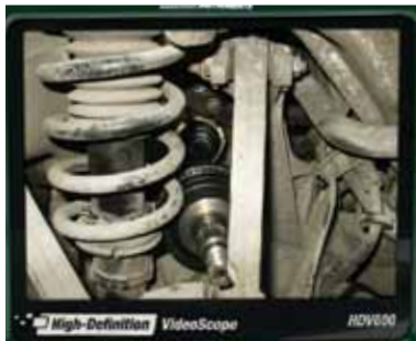
Features a 5.7" (144mm) high definition color LCD monitor
