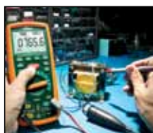
Measure the insulation resistance of transformer windings
