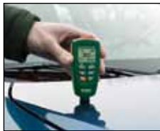
Measuring the thickness of automotive paint
